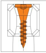
Brilliant design: the diameter of the eye is smaller than the wedge bolt, so the head cannot fly off.
